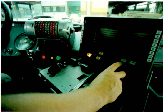
A Digital PDP-11/70 computer summons buses for customers of the RUFBUS system in Friedrichshafen, Germany, sells them tickets and tells them the number and arrival time of the bus. Simultaneously, aboard the buses in the system, a video display tells drivers how many riders are waiting and where they are located. This automated dial-a-ride system, the first in Germany, was developed by Dornier GmbH with the support of the German Ministry of Science and Technology.
