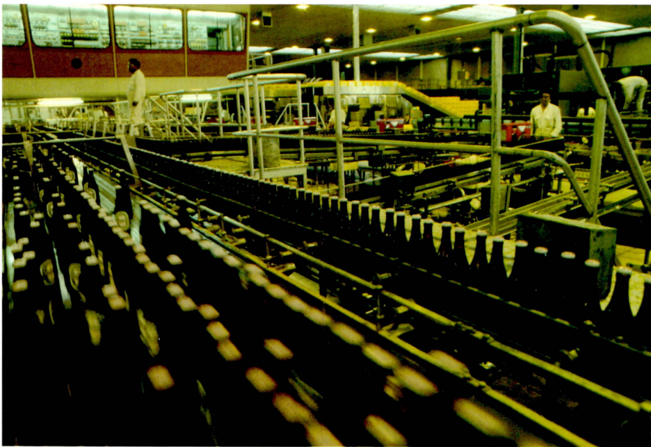
At the Heineken Brewery at Zoeterwoude, one of four operated by the famous Dutch Brewers in Holland, Digital PDP-11 computers are distributed throughout the automated bottling process to control the hourly production of 150,000 bottles of beer. A PDP-11/34 in the Heineken administrative office is used to develop software for the process control computers.
